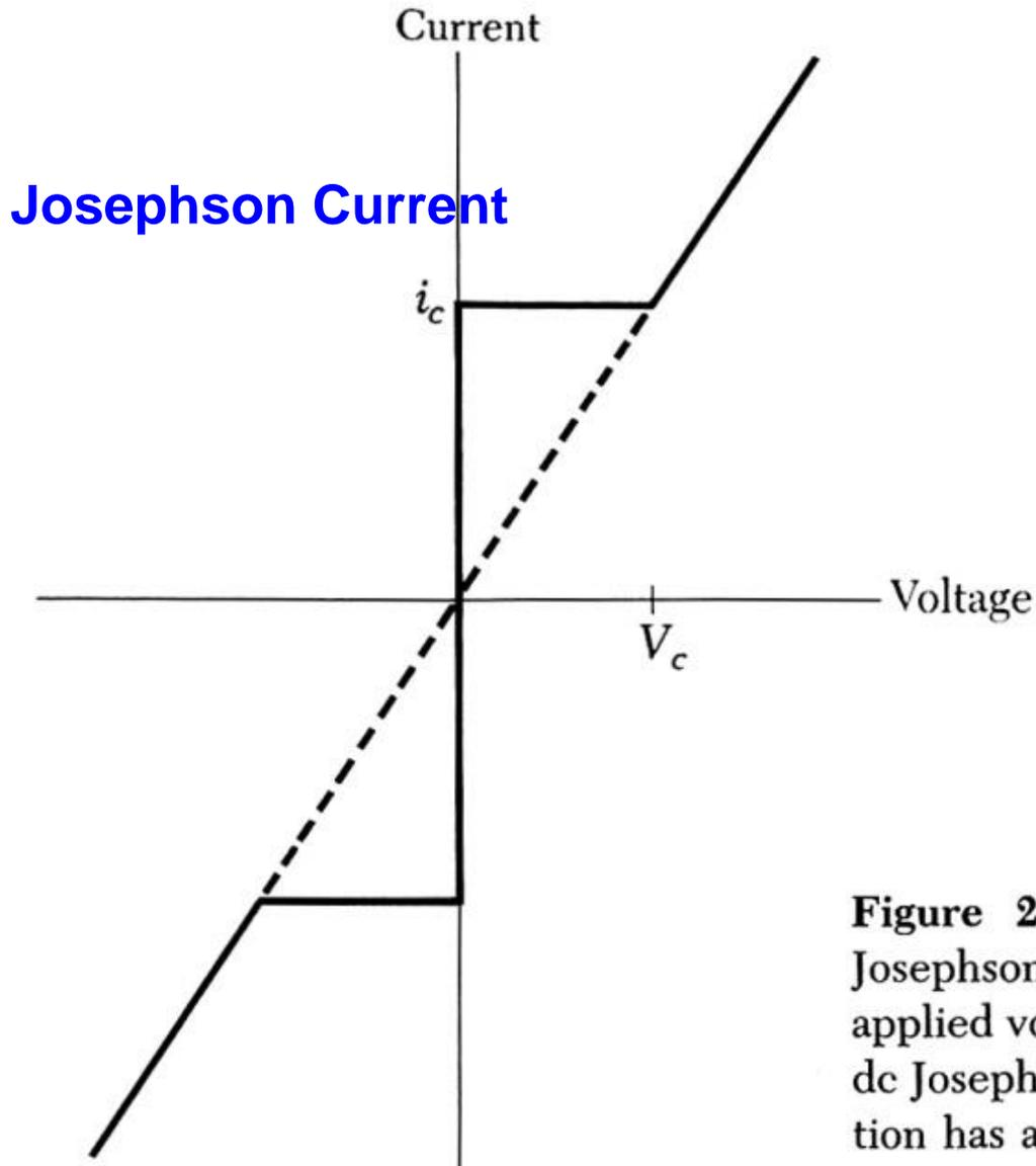
**Figure 24** Current-voltage characteristic of a Josephson junction. Dc currents flow under zero applied voltage up to a critical current  $i_c$ : this is the dc Josephson effect. At voltages above  $V_c$  the junction has a finite resistance, but the current has an oscillatory component of frequency  $\omega = 2eV/\hbar$ : this is the ac Josephson effect.
