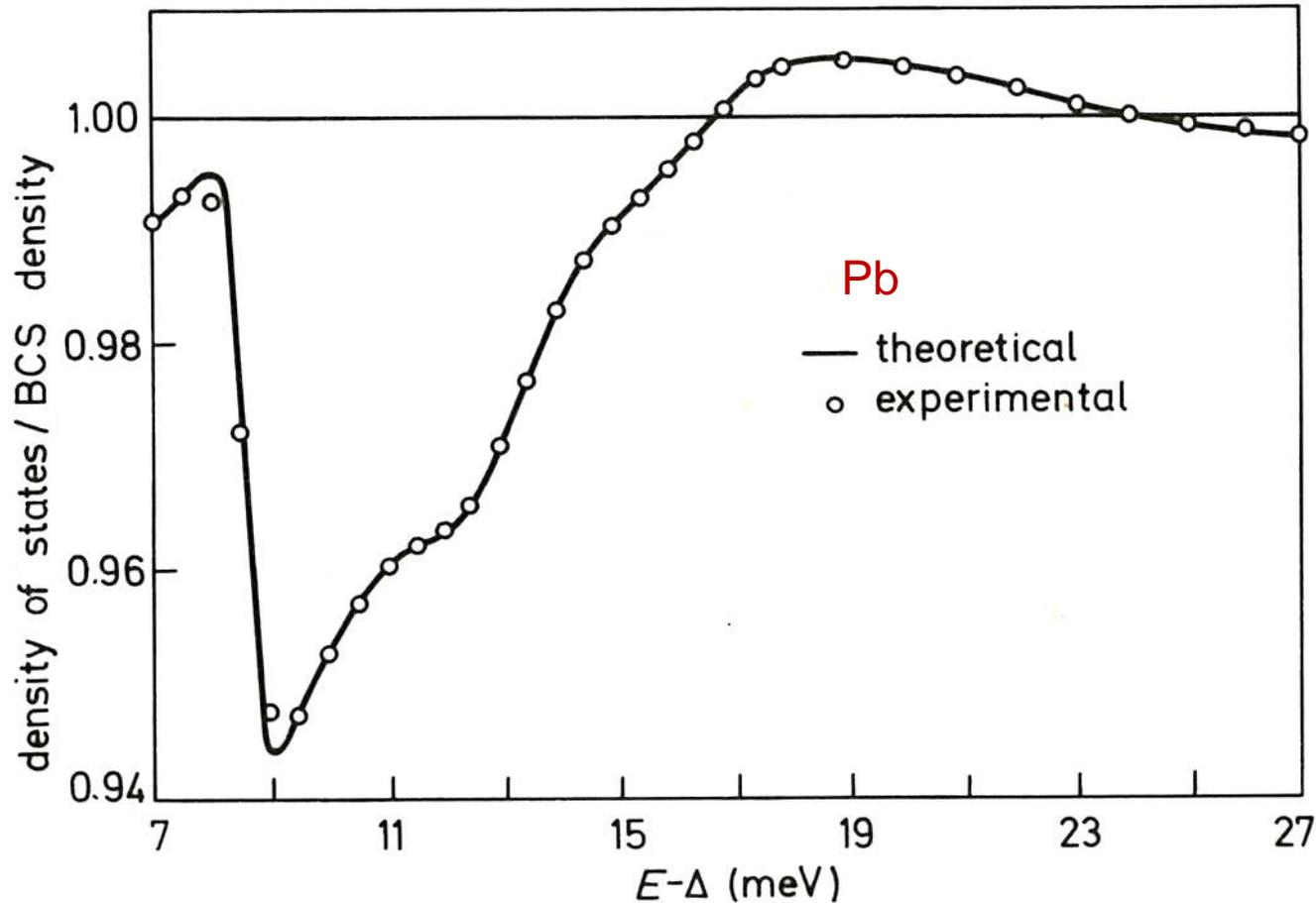
*Fig. 6.22* The density of states for lead related to the BCS density of states as a function of energy (zero shifted by  $\Delta$ ). In the experiment the sharp drop near 9 meV is affected by thermal smearing. After McMillan and Rowell [165].
