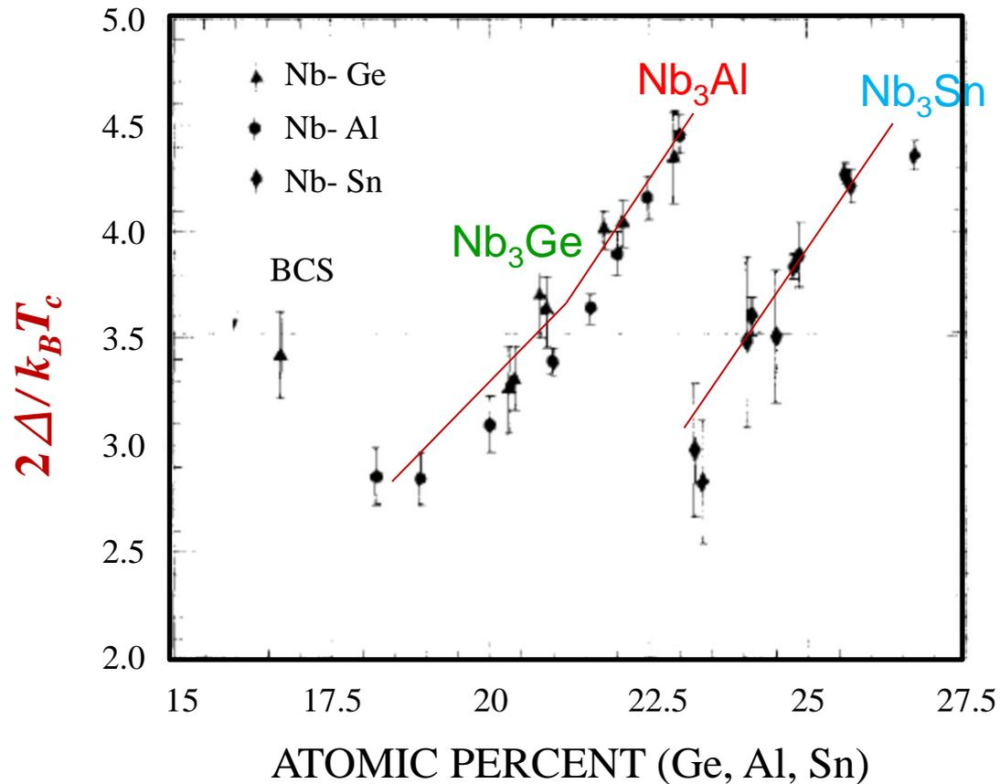
The variation with composition of the electron-phonon coupling strength  $2\Delta/k_B T_c$  for the A15  $Nb_3Sn$ ,  $Nb_3Al$ . And  $Nb_3Ge$ .
