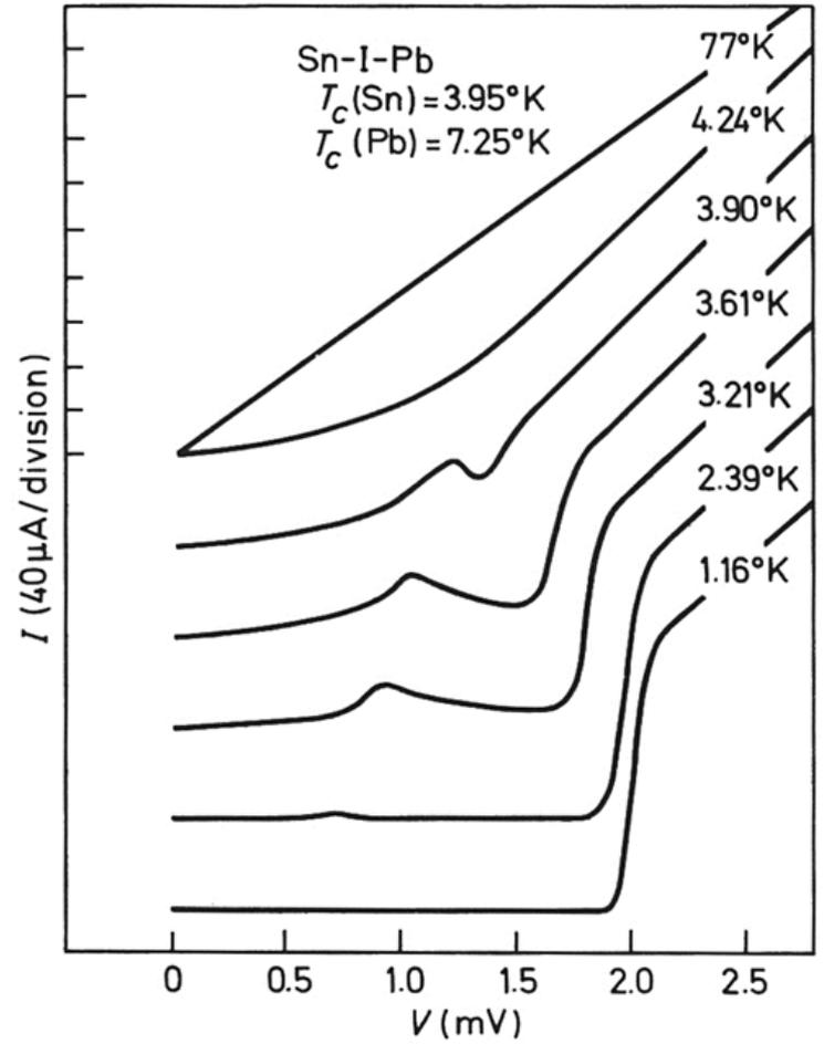
Fig. 4.9  $I$ - $V$  characteristics of an Sn-I-Pb junction.
