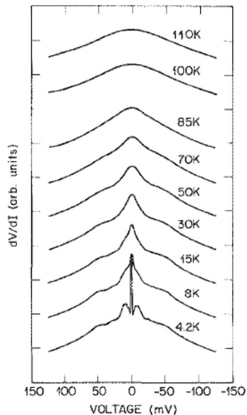
FIG. 2. Dynamic resistance  $R(V)$  vs  $V$  as a function of temperature below and above  $T_c$  of a  $Y_{1-x}Ba_xCu_3O_{7-x}$  film. The zero of  $R(V)$  at 4.2 K is on the base line, and the zeros of other traces are displaced progressively by one division.
