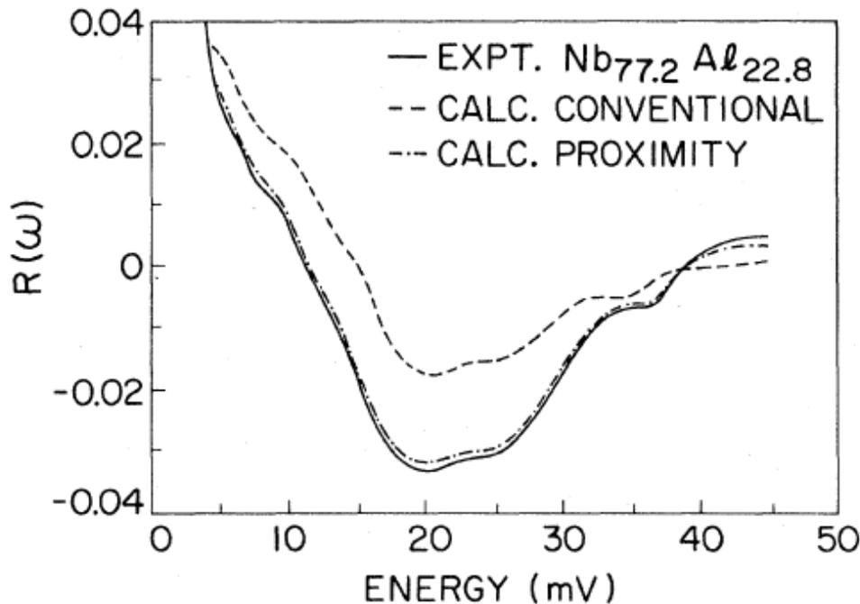
The experimental and calculated tunneling densities of states  $R(\omega)$ 's from both conventional (MR) and proximity inversion (MMR) analysis for the A15 Nb-Al junction of 22.8 at. % Al with  $T_c = 16.4$  K,  $\Delta = 3.15$  meV.
