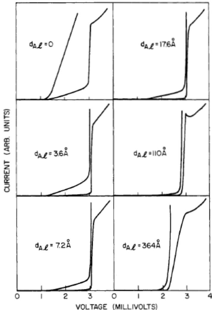
Fig. 2 Volt-ampere characteristics of Nb/Al-oxide-Pb<sub>0.90</sub>Bi<sub>0.10</sub> junctions with different  $d_{Al}$  at  $T = 2^{\circ}K$ . Expansion of the current scale  $\times 10$  is also shown. The junction without an Al overlayer was oxidized for 4 days, the rest for 20 min. All junctions have area  $S \approx 2 \cdot 10^{-3} \text{ cm}^2$ .
