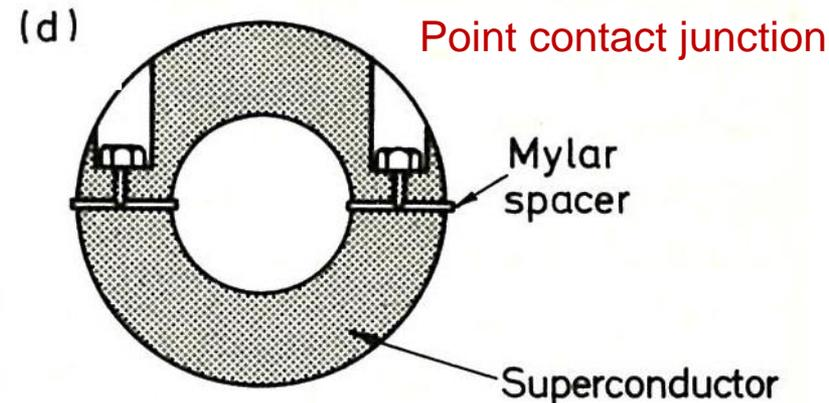
*Fig. 8.6* Weak links exhibiting properties similar to those of Josephson junctions. (a) A superconducting thin film bridge (Dayem bridge), (b) a superconducting thin film bridge with a normal metal overlay (Notary's bridge), (c) Clarke's solder drop junction (d) double point-contact junction developed by Zimmerman and Silver [341].
