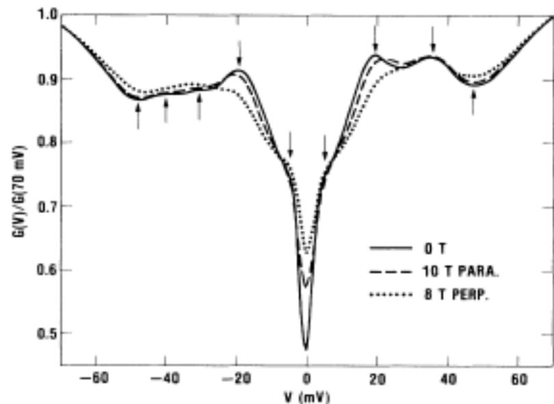
FIG. 2.  $G(V)$  for  $\text{YBa}_2\text{Cu}_3\text{O}_7/\text{Pb}$  junction in 0 T (solid line), 10.0 T (dashed line), and 8.0 T (dotted line) magnetic fields at  $T = 10 \text{ K}$ . Arrows indicate features which are discussed in the text.
