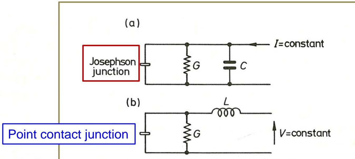
Fig. 11.1 Circuit representations of real junctions. (a) Thin film tunnel junction made up by an 'ideal' Josephson junction (satisfying the  $I = I_J \sin \phi$  relationship), an ohmic conductance and a capacitance; analysed for a constant current input. (b) An approximation to a point-contact junction taking account of parallel conductance and series inductance; analysed for a constant voltage input.
