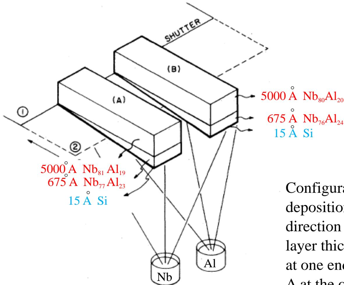
Configuration for the self-epitaxy deposition in the constant phase direction at  $950^\circ\text{C}$ . The epitaxial layer thickness is varying from zero at one end of the ten substrates to 675 Å at the other end.
