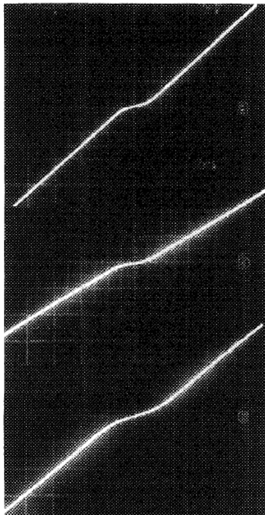
FIG. 1. Current-voltage characteristics for junctions (a), (b), and (c) at 4.2 K. The  $x$  axis (voltage) scales are 2, 2, and 1 mV per large division (pld) for (a), (b), and (c), respectively. The  $y$  axis (current) scales are 100, 250, and 250  $\mu$ A pld for (a), (b), and (c), respectively.
