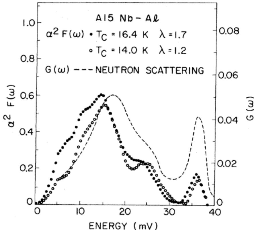
The electron phonon spectral functions  $\alpha^2 F(\omega)$  for two Nb-Al junctions with  $2\Delta/kBT_c$  of 3.6 and 4.4. The data of the neutron scattering function  $G(\omega)$  are after Schweiss *et al.*
