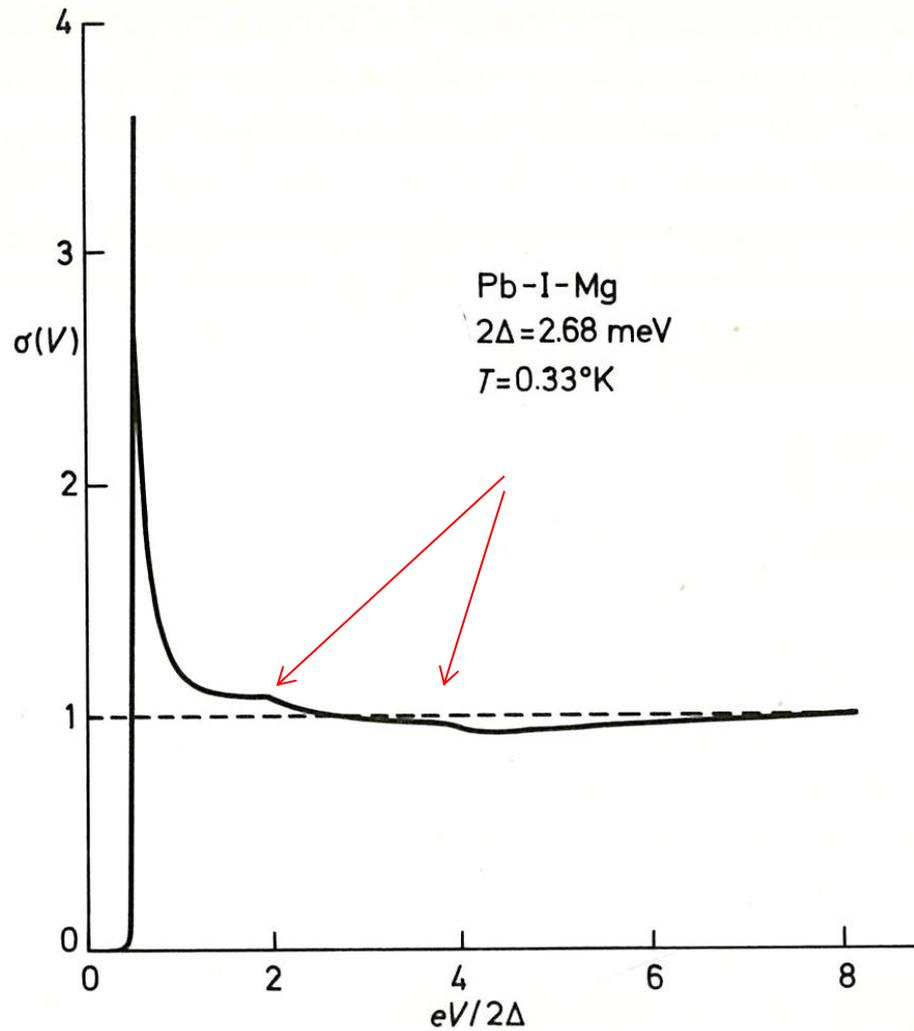
*Fig. 6.18* Normalised differential conductance as a function of normalised voltage for a Pb-I-Mg junction. The structure shown in the curve signifies deviation from the BCS theory. The cross-over point corresponds to the Debye energy. After Giaever, Hart and Megerle [66].
