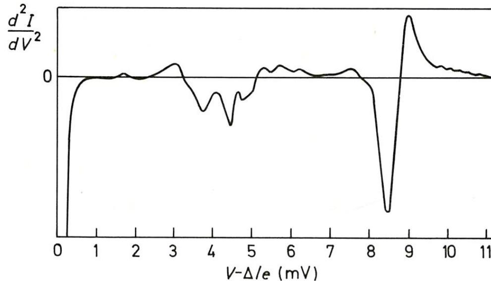
*Fig. 6.21* The second derivative of the  $I$ – $V$  characteristic as a function of voltage (zero shifted by  $\Delta/e$ ). Arrows indicate the voltage for Van Hove singularities on the basis of the neutron diffraction experiments of Brockhouse *et al.* [222]. After Rowell, Anderson and Thomas [221].
