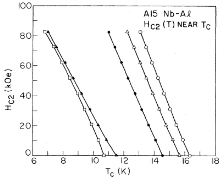
FIG. 1. Representative critical-field data near  $T_c$  of a series of A15 Nb-Al films measured. The lines drawn through data points are intended to serve only as a guide to the eye.
