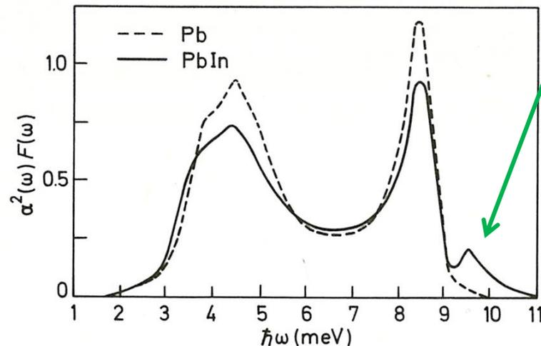
Fig. 6.23 The phonon spectrum  $\alpha^2(\omega)F(\omega)$  obtained by the gap inversion technique. The localised phonon mode of the light indium impurity may be seen at about 9.5 meV. After Rowell, McMillan and Anderson [227].
