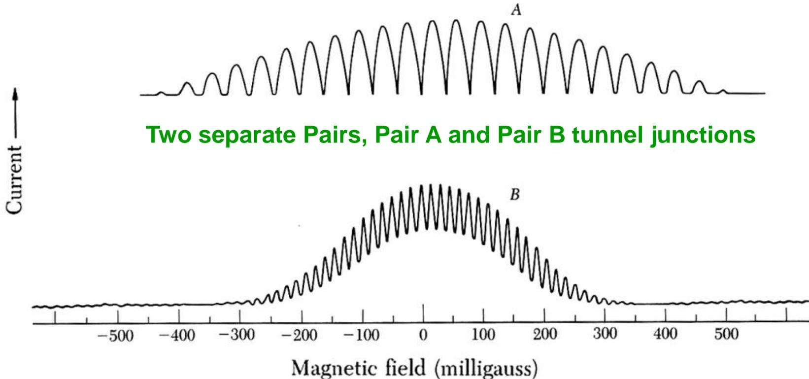
**Figure 26** Experimental trace of  $J_{\max}$  versus magnetic field showing interference and diffraction effects for two junctions A and B. The field periodicity is 39.5 and 16 mG for A and B, respectively. Approximate maximum currents are 1 mA (A) and 0.5 mA (B). The junction separation is 3 mm and junction width 0.5 mm for both cases. The zero offset of A is due to a background magnetic field. (After R. C. Jaklevic, J. Lambe, J. E. Mercereau and A. H. Silver.)
