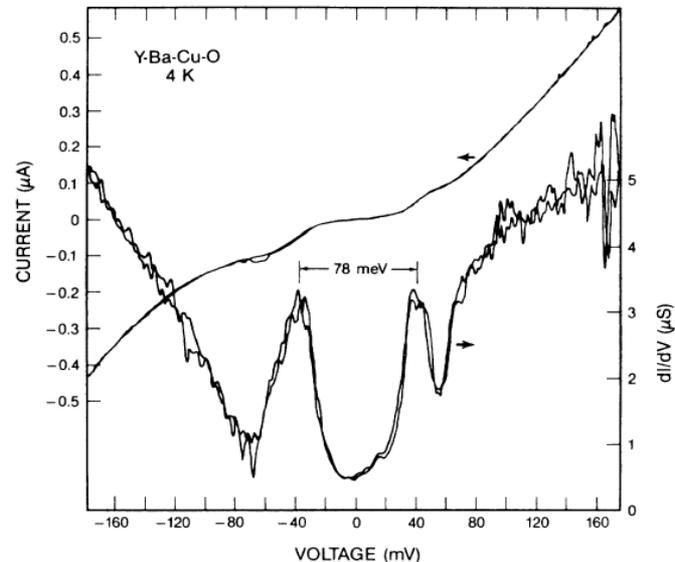
FIG. 2. Current-voltage characteristic and dynamic conductance ( $dI/dV$ ) showing superconducting gap structure typical of the largest measured in the  $Y_1Ba_2Cu_3O_{9-\delta}$  break-junction sample.
