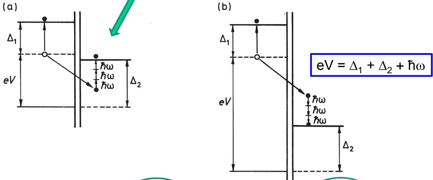
Fig. 5.7 Tunnelling assisted (a) by **absorption** of three photons, (b) by **emission** of three photons.
