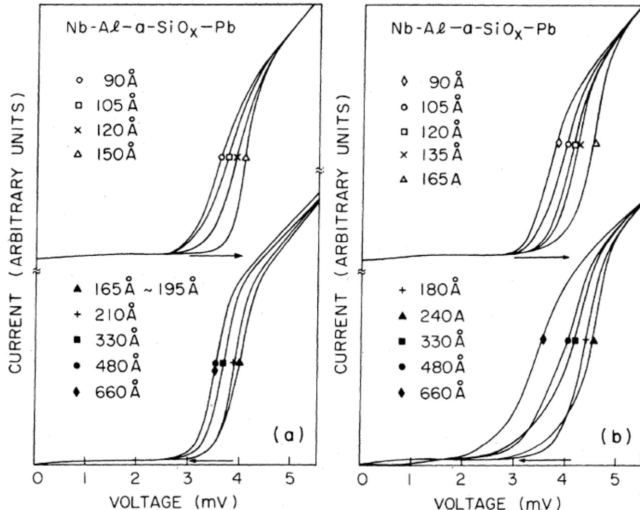
(a) Current vs voltage at 4.2 K of a series of tunnel junctions on the (A)-row self-epitaxial samples with epilayer thickness  $d$  systematically increasing from 90 to 660 Å. The composition of the epilayer is of 23 at. % Al. (b) The same for the (B)-row self-epitaxial sample. The composition of the epilayer is of 24 at. % Al.
