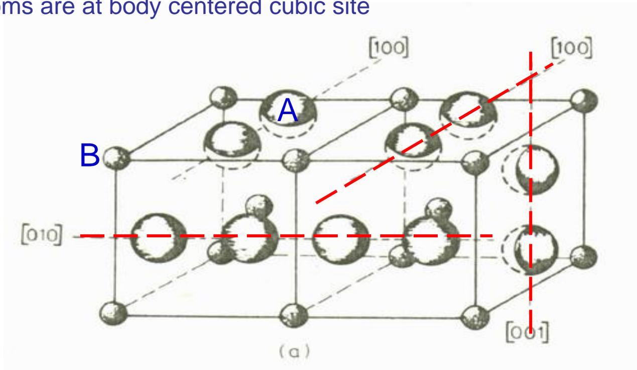
Fig. 34. (a) The position of A and B atoms in the unit cell of an  $A_3B$  compound possessing the  $\beta$ -W structure. (b) The Fermi surface of an  $A_3B$  compound in the tight binding, nearest neighbors approximation. There are three degenerate bands corresponding to electrons localized on the three families of chains.
