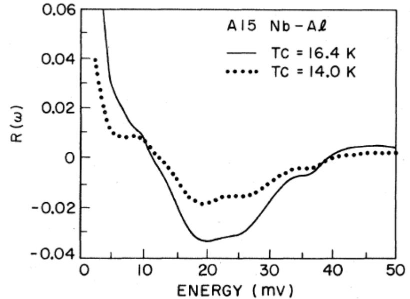
Reduced tunneling density of states  $R(\omega)$  vs energy above the gap for the two Nb-Al junctions of  $T_c = 16.4$  K,  $\Delta = 3.15$  meV, and  $T_c = 14.0$  K,  $\Delta = 2.15$  meV, respectively.
