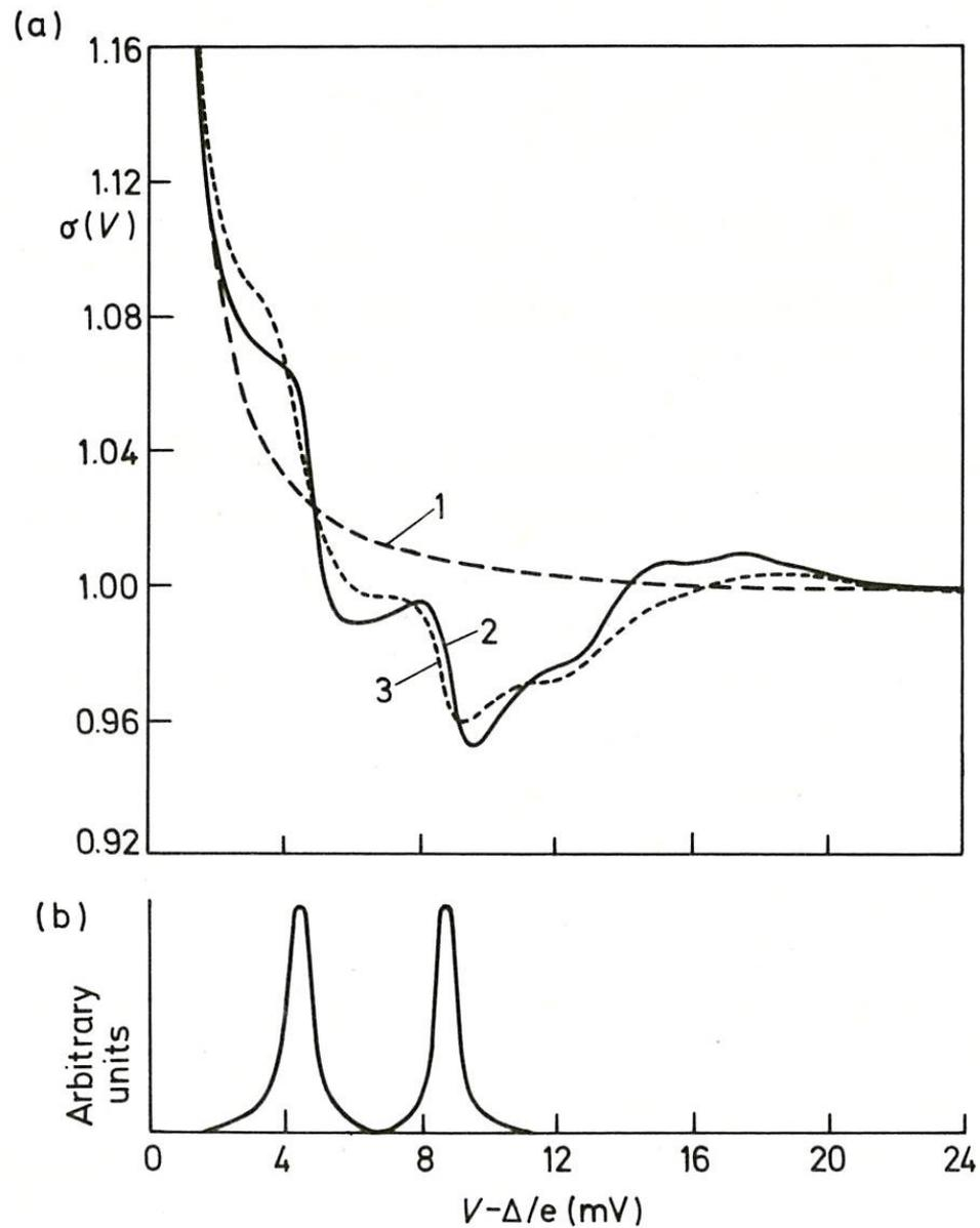
Fig. 6.20 (a) The normalised differential conductance as a function of voltage (zero shifted by  $\Delta/e$ ), 1: BCS theory, 2: theory by Schrieffer *et al.* [220], 3: experimental results by Rowell, Anderson and Thomas [221]. (b) The phonon spectrum assumed by Schrieffer *et al.* [220].
