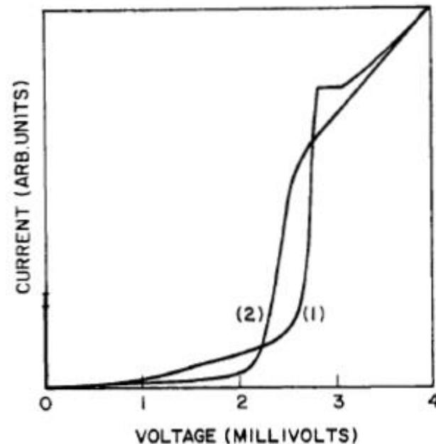
Fig. 3 Volt-ampere characteristics of Nb/Al-oxide-Nb (curve 1) and Nb/Al-oxide-Al/Nb (curve 2) junctions at  $T \approx 2^{\circ}K$ . Both base electrodes have  $d_{Al} = 25 \text{ \AA}$ , the top electrode of the junction with the second Al layer has  $d_{Al} = 32 \text{ \AA}$ . Critical currents are  $\sim 50 \text{ A/cm}^2$ .
