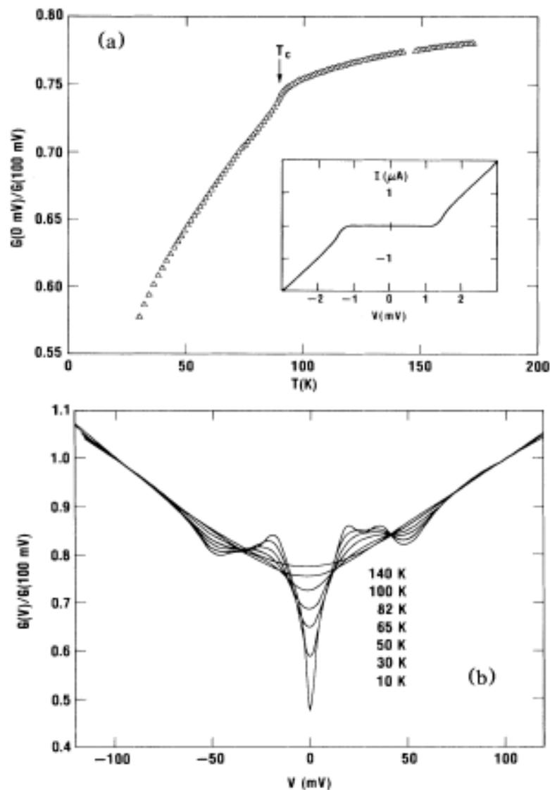
FIG. 1. (a) Temperature dependence of  $G(0 \text{ mV})/G(100 \text{ mV})$  of a  $\text{YBa}_2\text{Cu}_3\text{O}_7/\text{Pb}$  junction. Inset: Current vs voltage for a typical junction for  $T < 1 \text{ K}$ . Note the absence of leakage. (b) Voltage dependence of  $G(V)/G(100 \text{ mV})$  for the temperatures indicated for the junction in (a). The lowest-temperature curve has the lowest zero-bias conductance. The polarity refers to the  $\text{YBa}_2\text{Cu}_3\text{O}_7$  electrode.
