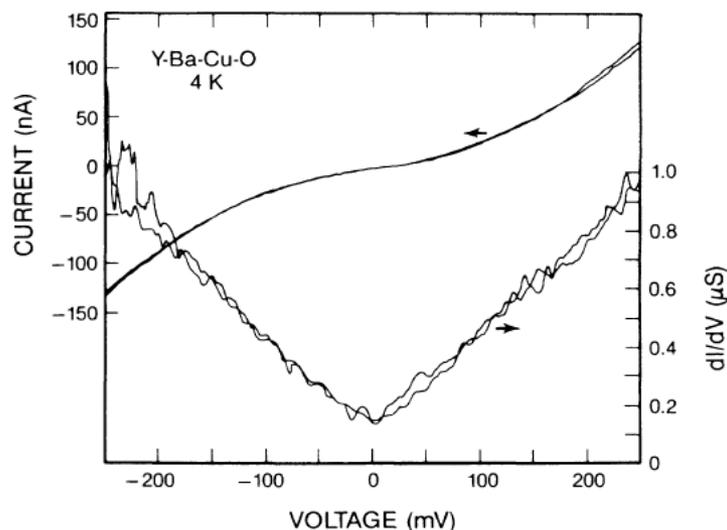
FIG. 1. Current-voltage characteristic and dynamic conductance ( $dI/dV$ ) characteristic of a  $Y_1Ba_2Cu_3O_{9-\delta}$  break junction immersed in liquid helium. This trace is typical of that predominately seen in the sample.
