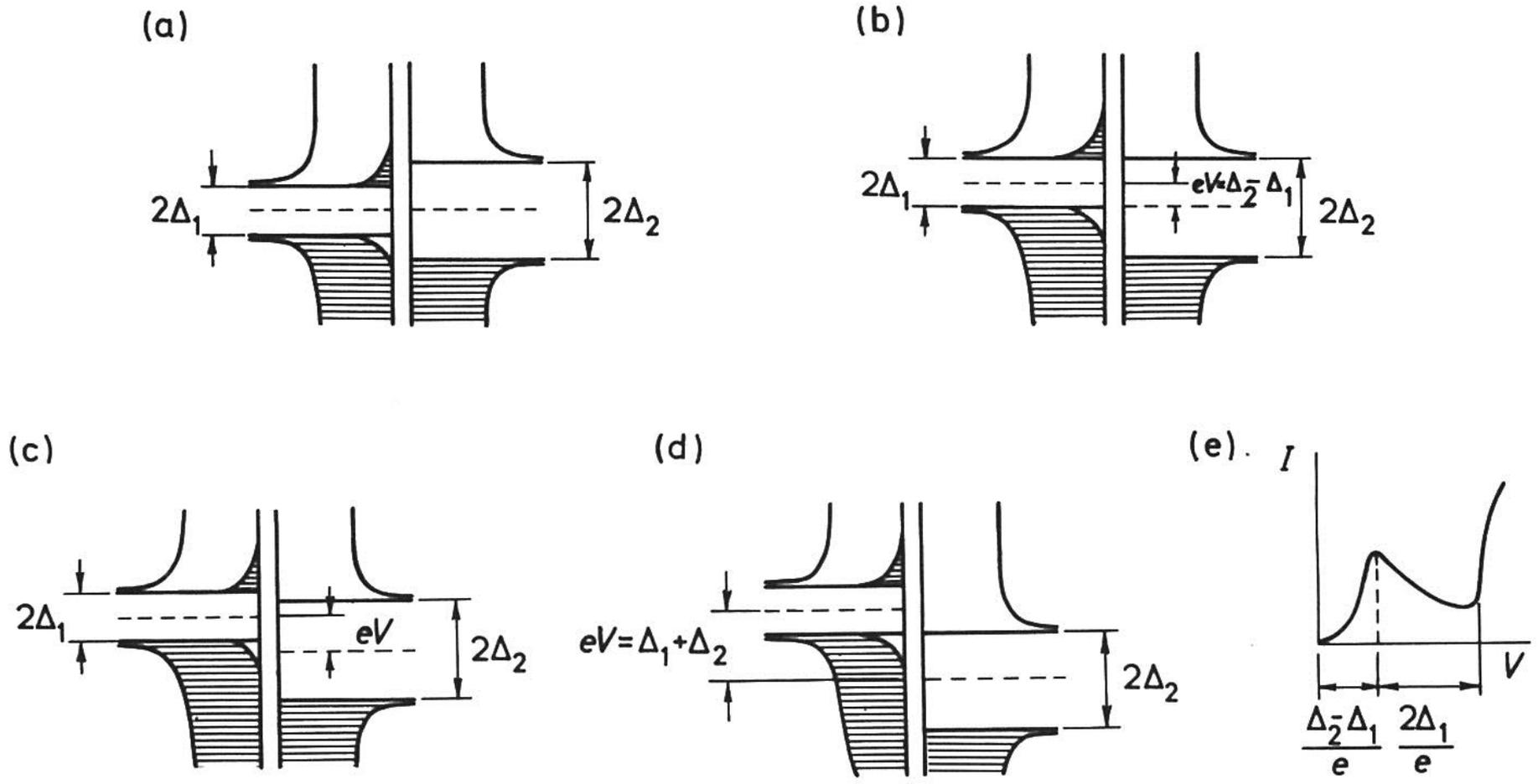
Fig. 4.7 The energy diagram and  $I-V$  characteristic of an  $S_1S_2$  junction at finite temperature; (a)  $V = 0$ , (b)  $V = (\Delta_2 - \Delta_1)/c$ , (c)  $(\Delta_2 - \Delta_1)/e < V < (\Delta_2 + \Delta_1)/e$ , (d)  $V = (\Delta_1 + \Delta_2)/e$ , (e) the  $I-V$  characteristic.
