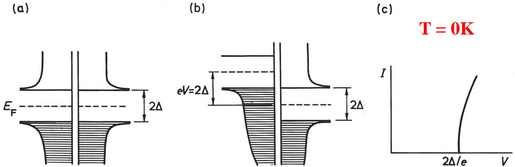
Fig. 4.4 The energy diagram of an SS junction; (a)  $V = 0$ , (b)  $V = 2\Delta/e$ , (c) the  $I$ - $V$  characteristic at  $T = 0$ .
