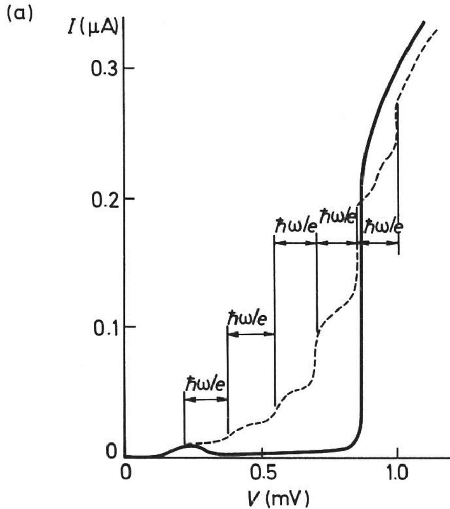
*Fig. 5.9 (a)*  $I$ - $V$  characteristic of an Al-I-In junction in the absence (solid lines) and presence (dotted lines) of microwaves of frequency 38.83 GHz. Measurements by Dayem and Martin, quoted by Tien and Gordon [58].
